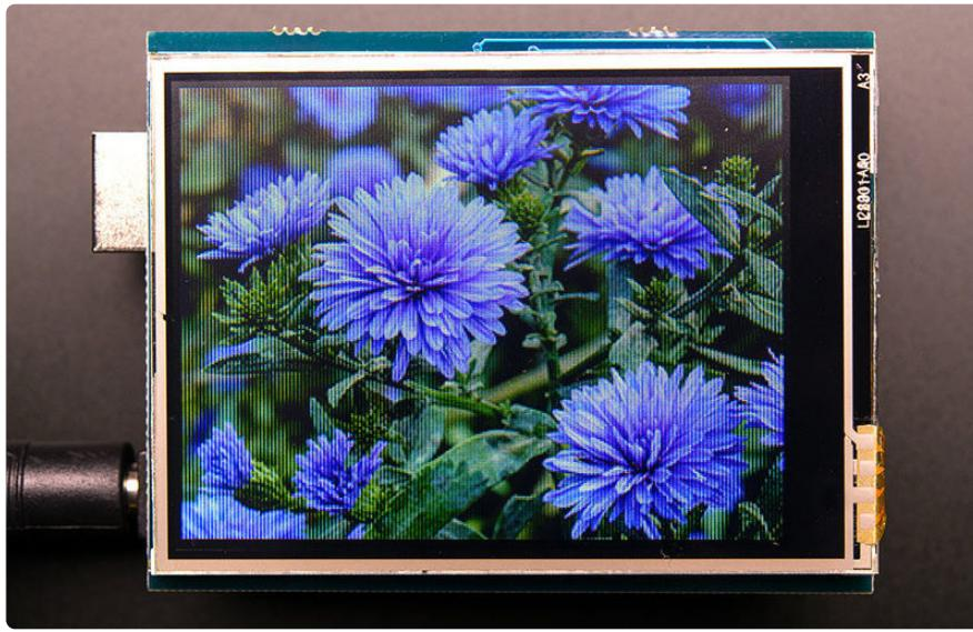
Loading .BMP images from an **SD card** (or the **flash memory chip** on Adafruit “Express” boards) is an option for most of our color displays...though it’s not built into Adafruit\_GFX and must be **separately installed**.
